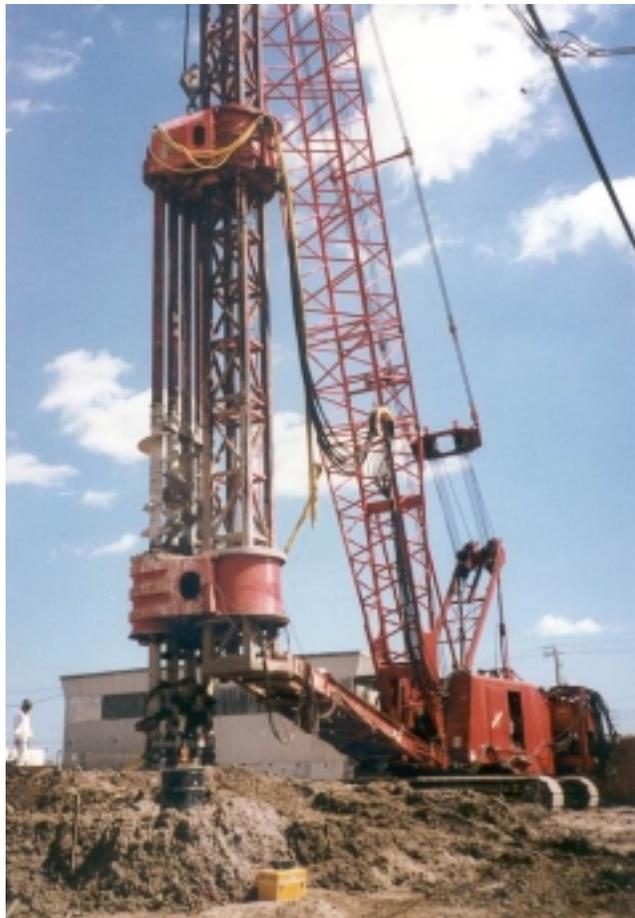
Figure 1. Deep Soil Mixing Drill Rig
