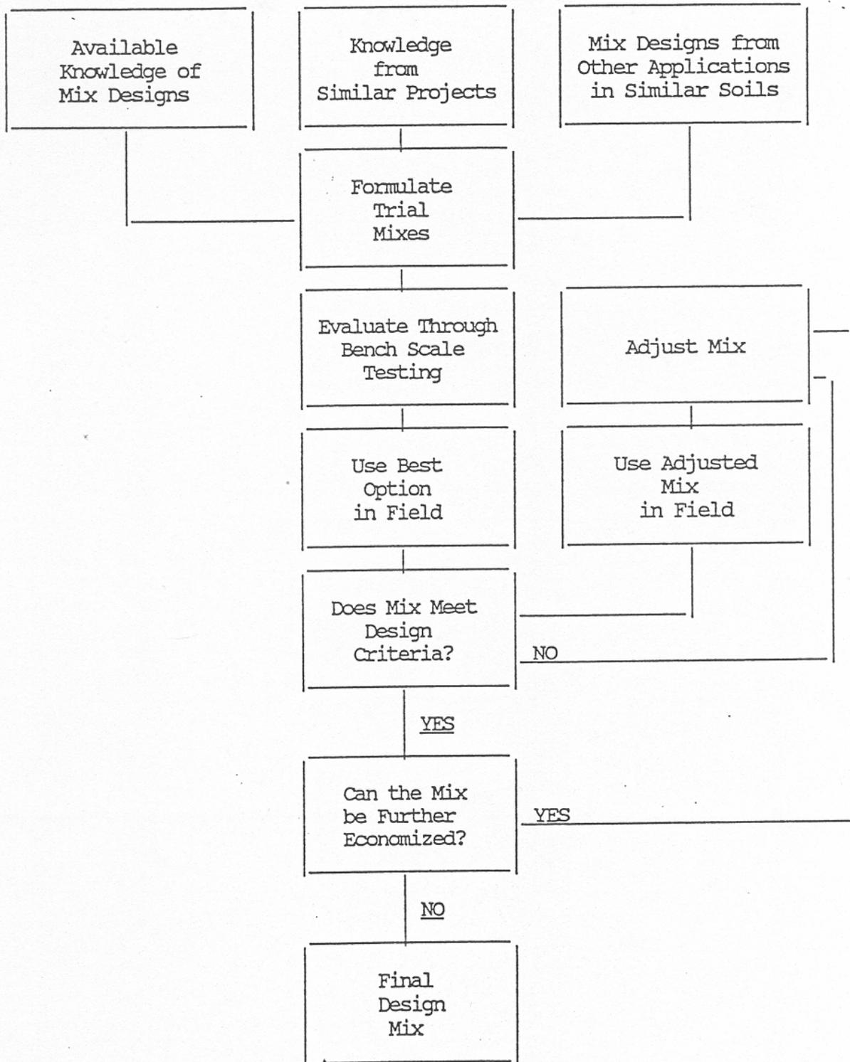
Especially for environmental applications, a preliminary mix design test can be performed to determine an optimum additive rate. This is very useful for applications when reductions in additive rates can be a major source of economy for the owner.
