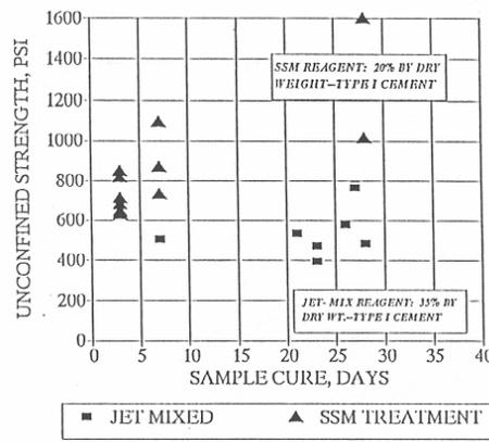
Figure 7. Soilcrete Strengths, Short Term
