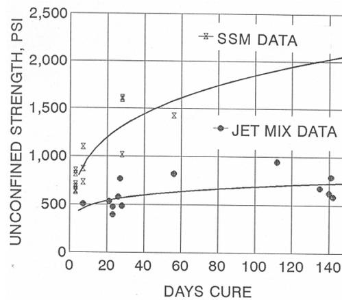
Figure 8. Soilcrete Strengths, Long Term
