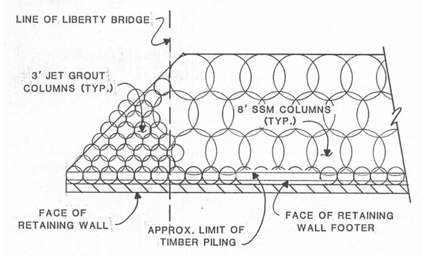
Figure 3. Layout of Soilcrete Columns
