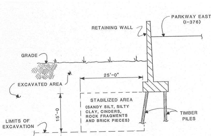
Figure 1. Cross Section of Stabilized Area
