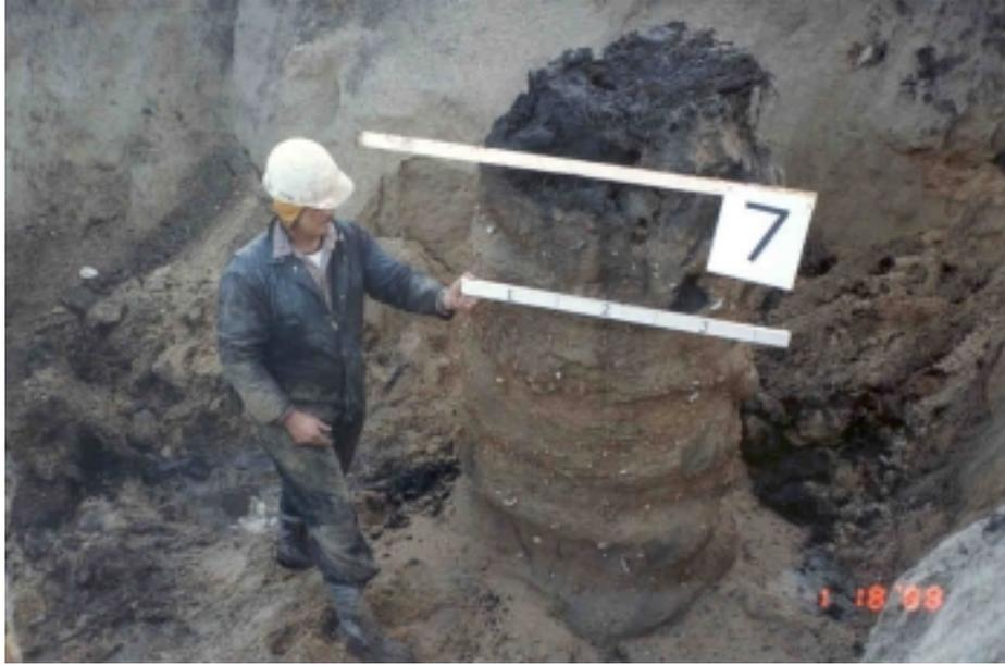
**Figure 5. Single Excavated Column from Test Program**
