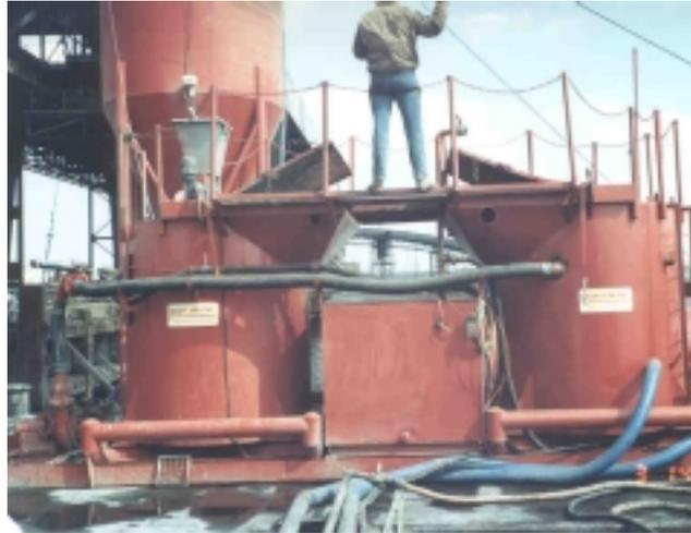
**Figure 8. Custom Built, Fully Automated Colloidal Mixing Plant**
