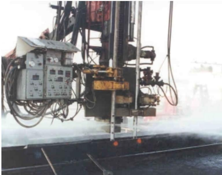
**Figure 10. Jet System and Control Panel**
