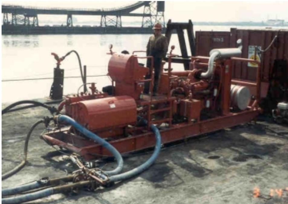
**Figure 9. High Pressure Triplex Piston Pumps**
