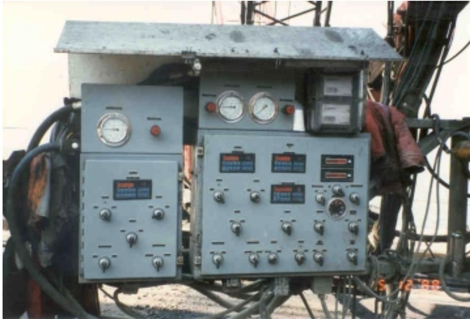
**Figure 11. Automated Drill and Extraction Controls**
