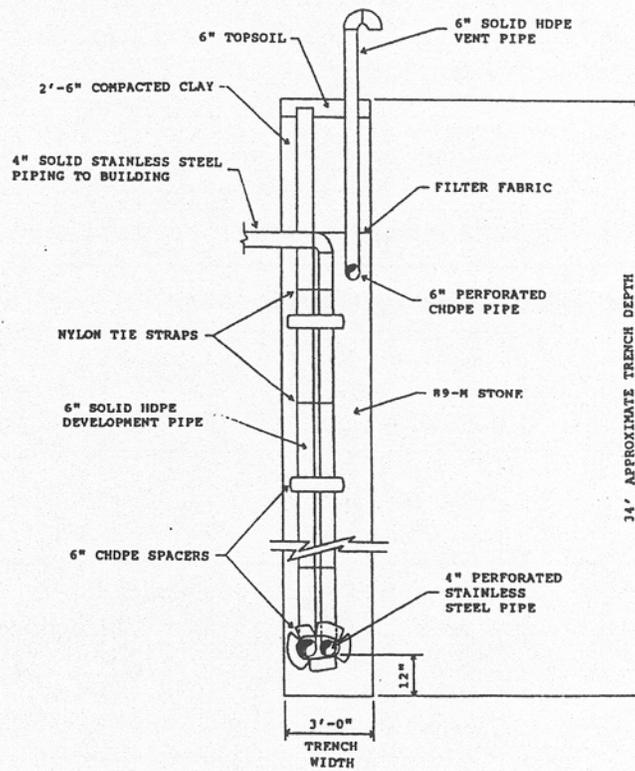
Figure 3: Typical trench cross section
