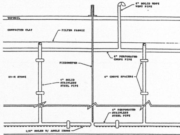
Figure 2: Typical trench section
