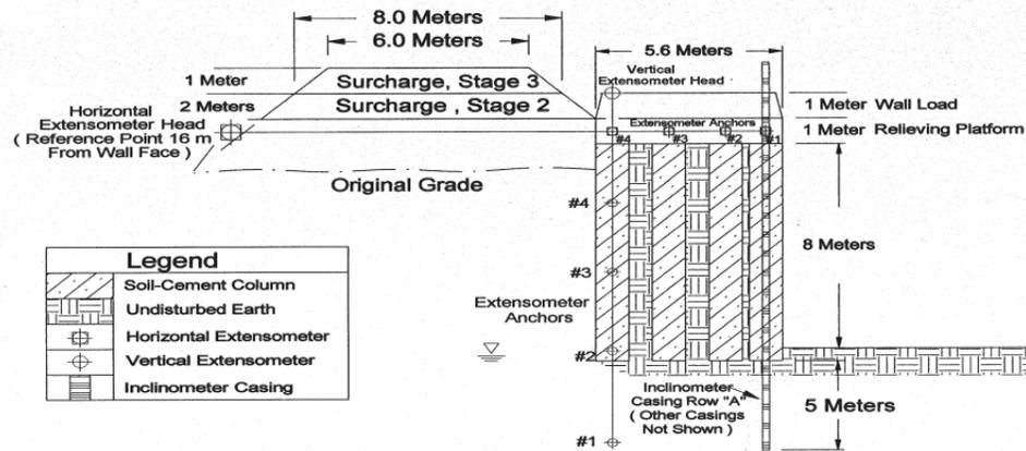
Figure 1. Cross Section of VERT Wall at College Station
