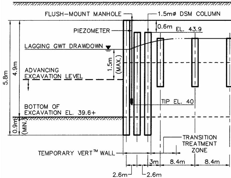
Figure 3 A Cross Section of Soil Cement Columns and VERT Wall Lakeland – Polk County, Florida
