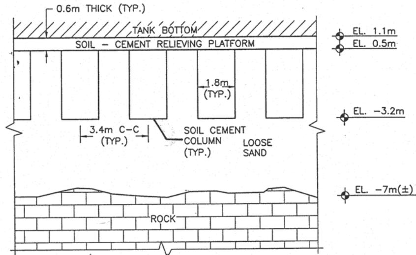
Figure 4. Cross Section of Soil Cement Columns at Honolulu, Hawaii
