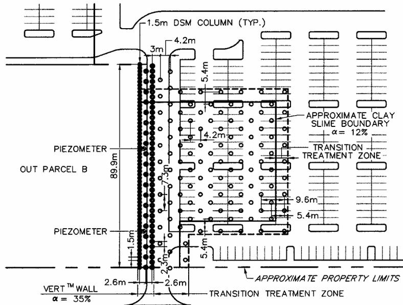
Figure 2. A Plan of Soil Cement Columns and VERT Wall Lakeland – Polk County, Florida
